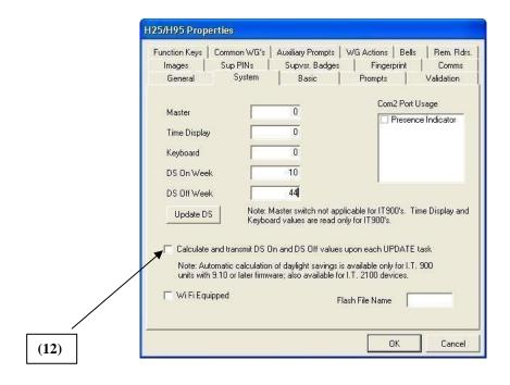
13. After making the above corrections, click the Comms tab and click the Transmit New Station Configuration button. Once done transmitting the information to the clock, select the OK button. Click OK again to close the station properties.
